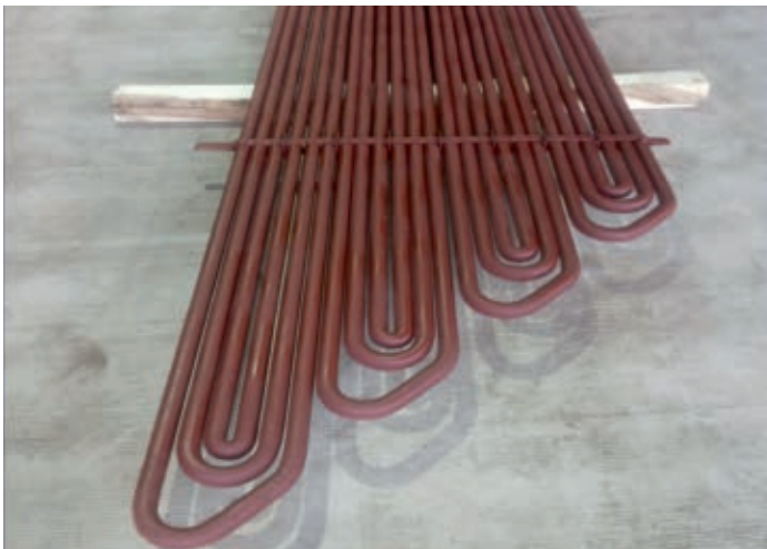
Super Heater Coils | SA 213, Gr T22, Alloy Steel
