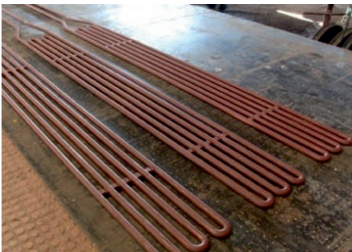
Super Heater Coils | SA 210, Gr A1, Carbon Steel
